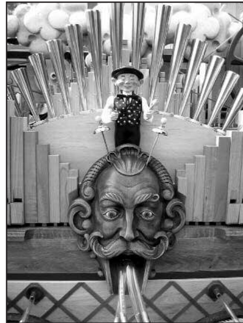
Figure 2. A close-up of the front of the organ details the "Kleien-Kotzer" whose mouth serves the purpose of being the entrance/exit of the pneumatic tubes used to activate the different functions.
